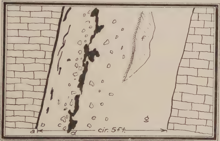
(24) Section of vein at a point on 145 ft. level, No. 3 shaft, Blue and Marble mine, Mexico district. a. band of fragmental spar, calcite, galena and rock; b. massive spar spotted and streaked with galena; c. spar with inclusions of calcite; d. zone of galena; e. spar with inclusions of calcite; f. rock; g. massive fluorspar.
